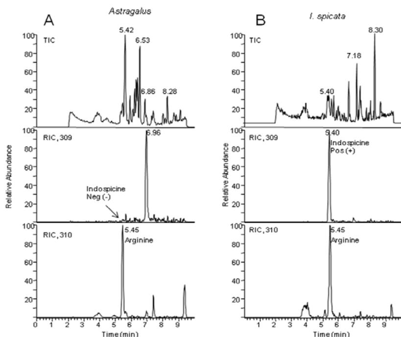
Figure 3. LC-esiMS analysis of *Astragalus* plant material (A) used for indospicine negative control and *Indigofera spicata* (B) used for indospicine positive control. Each sample includes the total ion chromatogram (TIC) and their reconstructed ion chromatograms for  $m/z$  309 (indospicine) and  $m/z$  310 (arginine).
