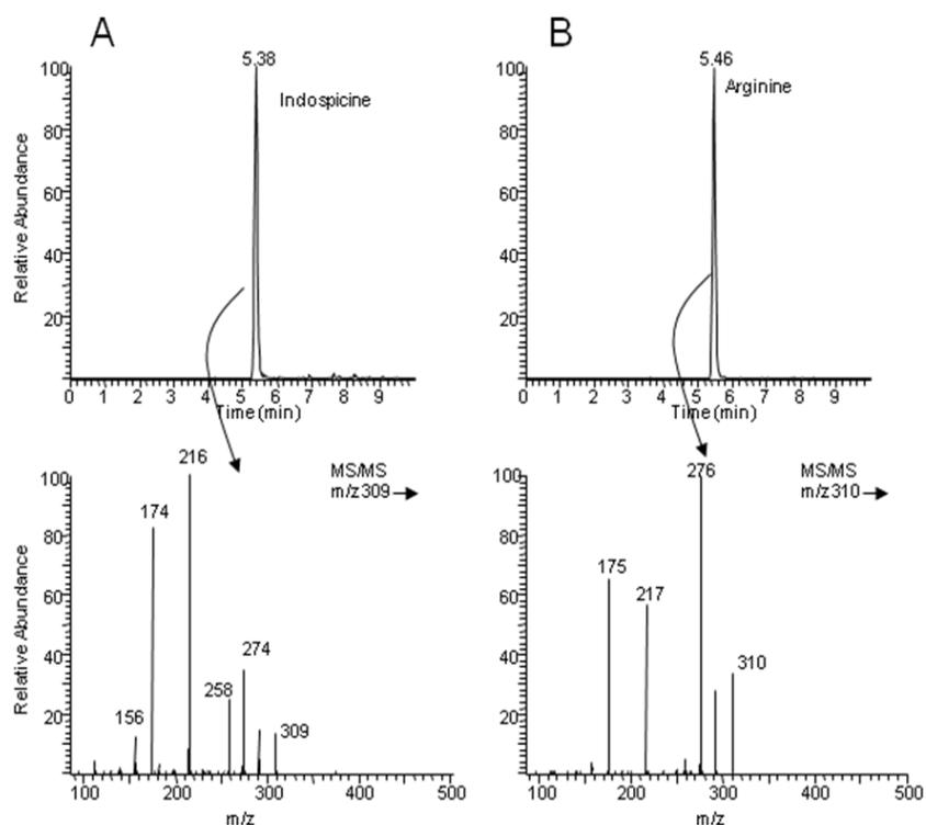
Figure 4. LC-esiMS/MS analysis of standard solutions of indospicine (A) and arginine (B) and their corresponding MS/MS spectra resulting from fragmentation of the parent ions for indospicine ( $MH^+ = 309$ ) and arginine ( $MH^+ = 310$ ).
