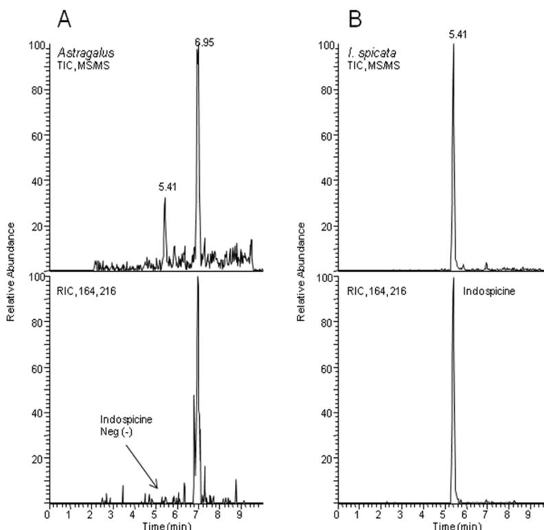
Figure 5. LC-esiMS/MS analysis of *Astragalus* plant material (A) used for indospicine negative control and *Indigofera spicata* (B) used for indospicine positive control. Each sample includes the total ion chromatogram (TIC) and the reconstructed ion chromatograms for  $m/z$  309  $\rightarrow$  174, 216 the selected ions for indospicine.
