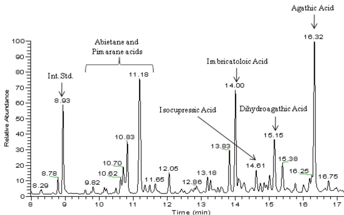
Figure 2. Chemical analysis of western juniper bark. Gas chromatography/mass spectrometry chromatograms and the major diterpene acids identified from the plant material. Specific peaks include Imbricatoloic Acid (Rt, 14.00 min), Isocupressic Acid (Rt, 14.61 min), Dihydroagathic Acid (Rt, 15.16 min), and Agathic Acid (Rt, 16.32 min).
